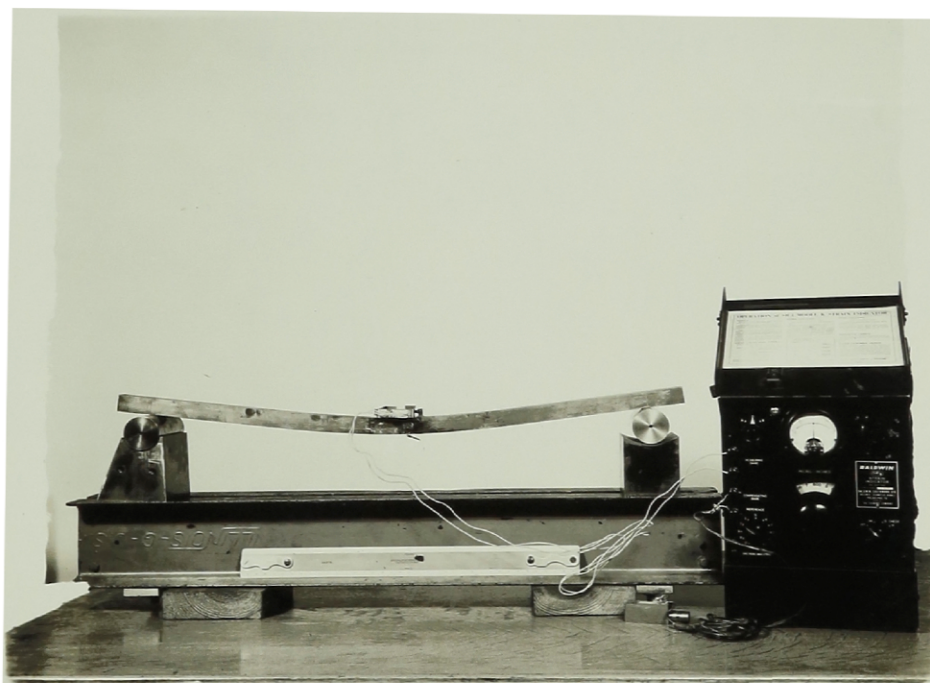
FIG.119 - CALIBRATION OF CLIP GAGE BY SR-4 GAGE
